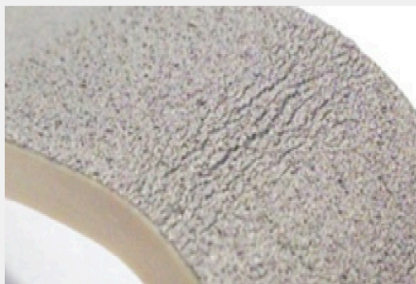
Figure 1: EN ISO 7438 bending tests of 6 plasma-spray-coated implant surfaces clearly show cracks in the coating layer. A further consequence may be delamination / abrasion. In-house research.
