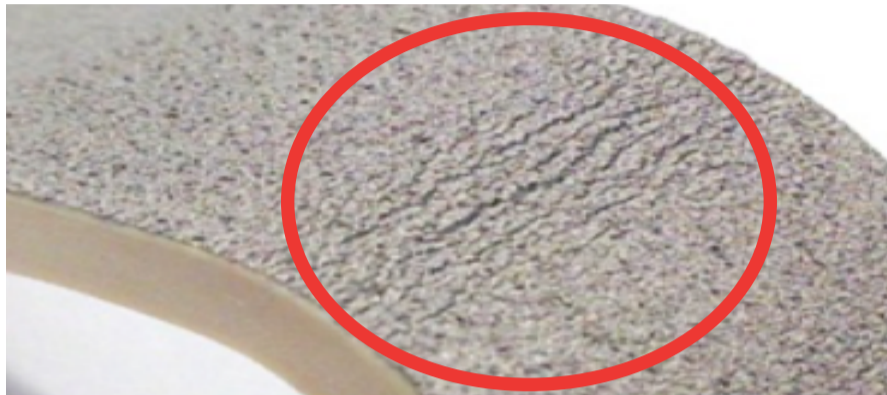
Picture 5,6: EN ISO 7438 TESTING of PLASMA SPRAY COATINGS. In-house research.
