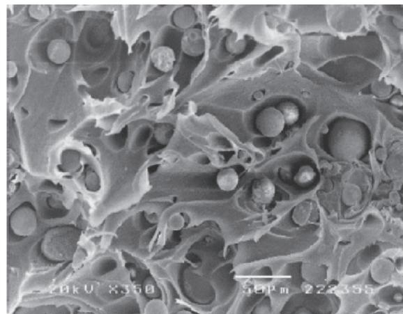
**Figure 2.** Scanning electron microscopy (SEM) micrograph of a PEEK-HA composite fracture area, demonstrating a debonding of the HA particles from the PEEK matrix. Reproduced with permission.<sup>[112]</sup> Copyright 2004, Elsevier. Scale bar: 50  $\mu$ m.
